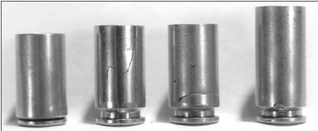
Left to right: case head collapsed into body; cracked wall; incipient blowout at feed ramp; extractor damage to web and rim.
